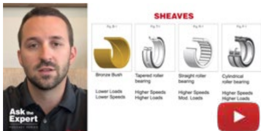
Ep. 27 Sheaves: bronze bushing vs roller bushing
